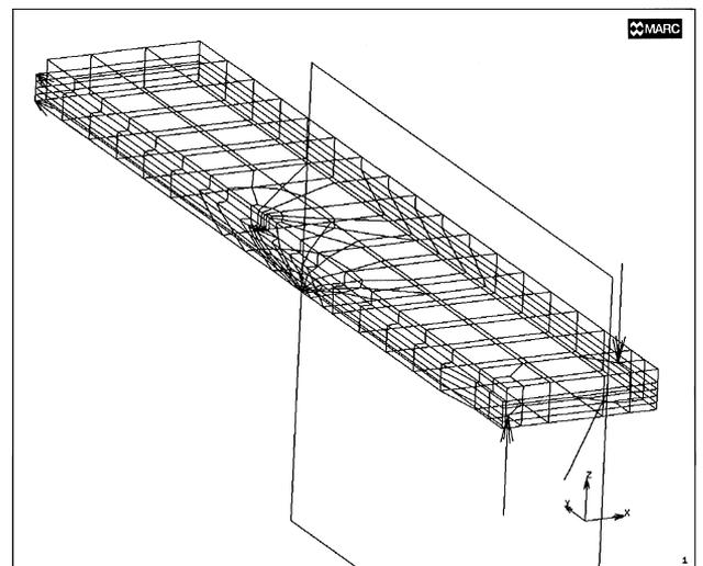
Fig. 2. The finite-element mesh. The model represents one half of a *DT* specimen. The remaining part is replaced by symmetry conditions and by a contact surface in the ruptured interface. The side-groove and initial notch are reproduced. The crack front is curved as observed in the experiments.
