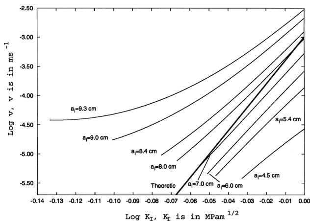
Fig. 7. The  $v-K_I$  curves obtained by applying Evans' analysis to some relaxation experiments simulated with the aid of the corrective curves for the Specimen 1. The initial load is the same for all experiments, the different values of the initial crack length are indicated for each curve.
