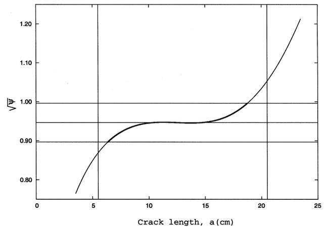
Fig. 6. The corrective function for  $K_I$  for the geometry called ‘Specimen 2’ ( $L = 25$  cm,  $W = 10$  cm,  $d = 7$  mm,  $d_n/d = 1$ ,  $g_w = 0$  mm,  $nl = 2$  cm,  $c = 4$ ). The vertical lines delimit the range explored in the present analysis. The horizontal lines define the operational range where  $K_I$  is constant within 5% (thick line).
