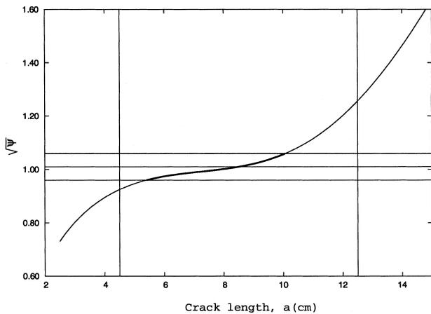
Fig. 5. The corrective function for  $K_I$  for the geometry called ‘Specimen 1’ ( $L = 17$  cm,  $W = 10$  cm,  $d = 7$  mm,  $d_n/d = 1/2$ ,  $g_w = 2$  mm,  $nl = 2$  cm,  $c = 4$ ). The vertical lines delimit the range explored in the present analysis. The horizontal lines define the operational range in which  $K_I$  is constant within 5% (thick line).
