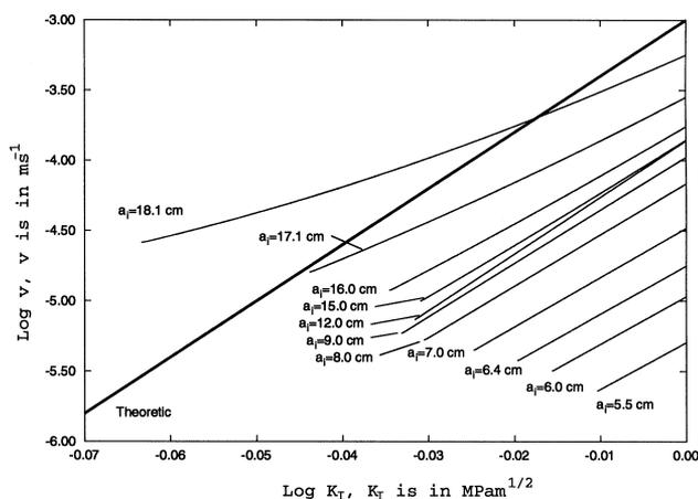
Fig. 8. The  $v-K_I$  curves obtained by applying Evans' analysis to some relaxation experiments simulated with the aid of the corrective curves for the Specimen 2. The initial load is the same for all experiments, the different values of the initial crack length are indicated for each curve.
