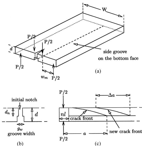
Fig. 1. The sketch of a double-torsion specimen: (a) general view, (b) axial cross-section, (c) longitudinal cross-section (modified after Atkinson [3]).
