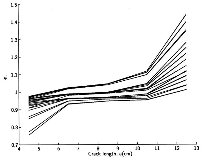
Fig. 4. The corrective coefficients of  $\psi$  for specimens with length  $L = 17$  cm and width  $W = 6$  cm. The different curves represent all combinations of the other geometric parameters.
