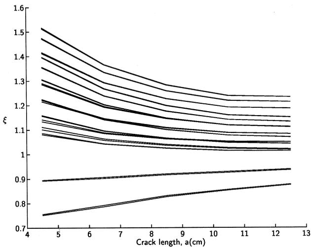
Fig. 3. The corrective coefficients of  $\zeta$  for specimens with length  $L = 17$  cm and width  $W = 6$  cm. The different curves represent all combinations of the other geometric parameters.
