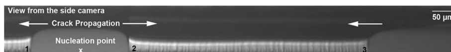
Fig. 4 Representative image of the observation from the side camera showing three crack-tips of Bg1110 against PMMA as the adhesive is separated from the substrate after applying a fixed imposed displacement. The crack-tips have been labelled as 1, 2 and 3 with the directions indicated by the arrows. The white region at the interface is a reflection of the light shined on the adhesive. The positions of the crack 2 and crack 3 have been traced and plotted as a function of time in Fig. 5.
